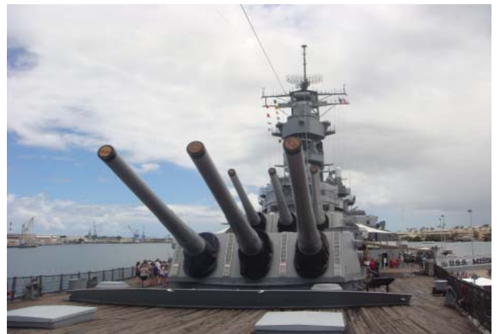
Mighty Mo’s trademark feature is her 16 inch guns. Each gun barrel is approximately 67 feet long, weighs 116 tons, and can accurately fire a 2,700–pound shell 23 miles in about one minute.
